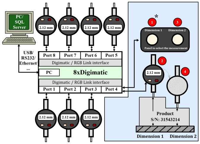
Fig. 2. Measurement of two dimensions of products using the control panel
