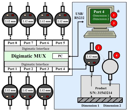
Fig. 1. Measurement of two dimensions of a product via PC
